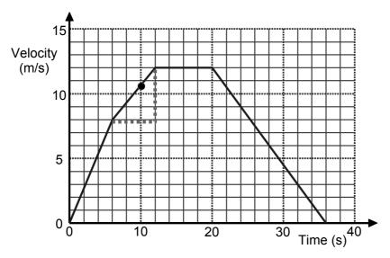
Acceleration = gradient of line =  $\frac{12-8}{12-6} = \frac{4}{6} = \frac{2}{3}$  m/s<sup>2</sup>
